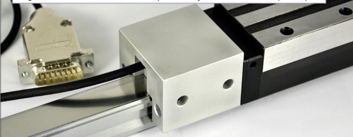
The measuring system is suitable for extreme service, the readhead have a sealing to IP68, and is highly resistant to shock, vibrations and pressure. The non-contact, frictionless design eliminates wear while reducing hysteresis giving precision at high speeds and accelerations.
